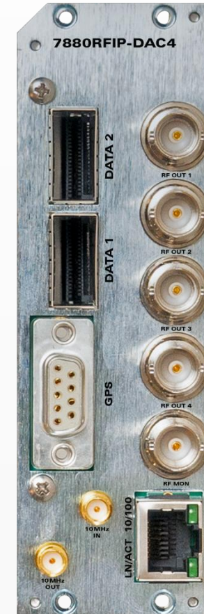
Quad IP to RF Conversion
